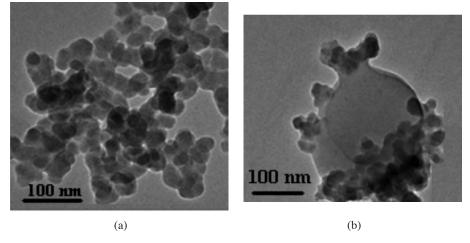
FIGURE 2. TEM images of (a)  $SiO_2$  NPs (b) PFO/SiO $_2$  nanocomposite (50 wt. %  $SiO_2$ )
