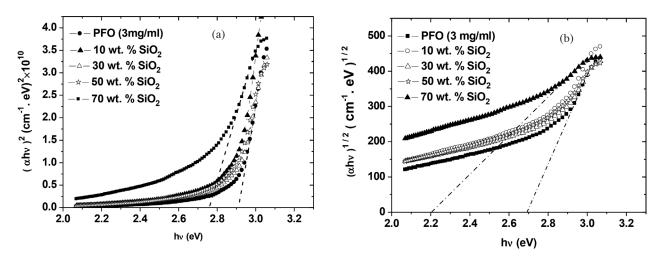
FIGURE 4. Dependence of (a):  $(\alpha hv)^2$  and (b):  $(\alpha hv)^{1/2}$  on photon energy (hv) for Pure PFO and PFO/SiO<sub>2</sub> nanocomposites
