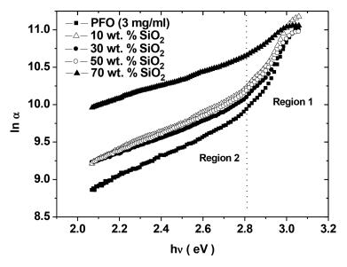
FIGURE 5. ln  $\alpha$  as a function of photon energy for PFO and PFO/SiO $_2$  nanocomposites
