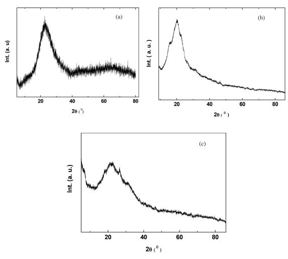
FIGURE 1. Typical XRD patterns for (a)  $SiO_2$  NPs, (b) Pure PFO and (c) PFO/50 wt.%  $SiO_2$  NPs
