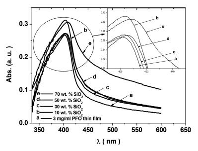
FIGURE 3. Absorption spectra for PFO and PFO/SiO2 nanocomposites
