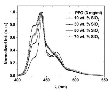
FIGURE 6. Normalized fluorescence intensity of pure PFO and PFO/  $SiO_2$  nanocomposite
